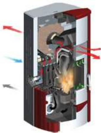
Special kinds of stoves have been constructed to combust only pelletized material. Pellet stoves are very popular and installed both in urban and rural areas. The stove components are much more sophisticated than the firewood stoves. An electric fan controls the combustion process by varying the supply of combustion air. This results in low CO and C<sub>x</sub>H<sub>y</sub> emissions.
