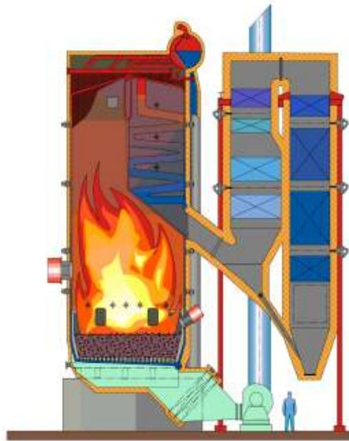
Fluidised bed boilers from 3,0 – 50 MW, max. pressure 100 bar (g), max. temp. 520°C, fuels: wood chips, wood waste, peat (Renewa Oy).
