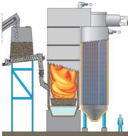
Heat-only boiler 3-50 MW, max. pressure 10-20 bar (g), max. temp. 120-200°C, fuels: wood, bark, forest desidues, peat (Renewa Oy).
