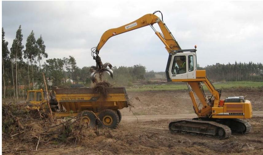
Figure 9. Elevating cabin improves the visibility and therefore the productivity.
