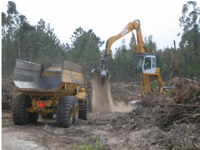
Figure 7. Tracked lifting machine is loading the dumper with split stumps and roots.
