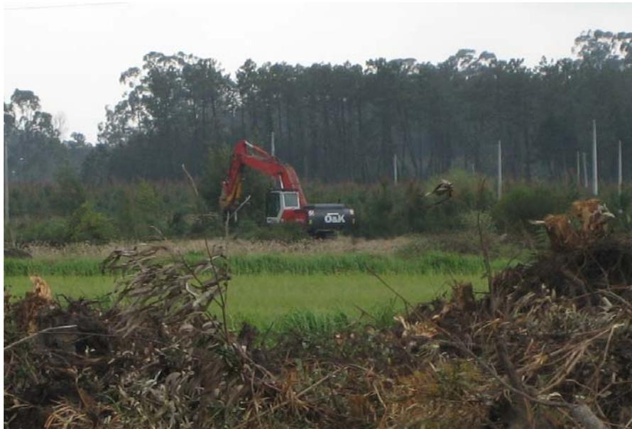
Figure 5. Stump and root lifting with a 28 tonne excavator in Portugal.
