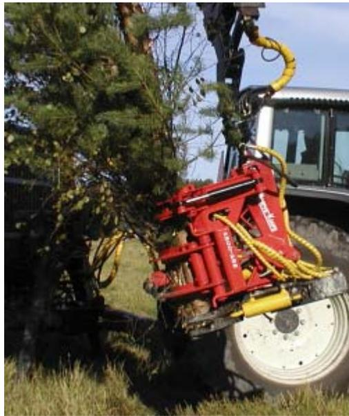
Figure 3. Naarva Grip accumulating felling head attached to farm-tractor.
