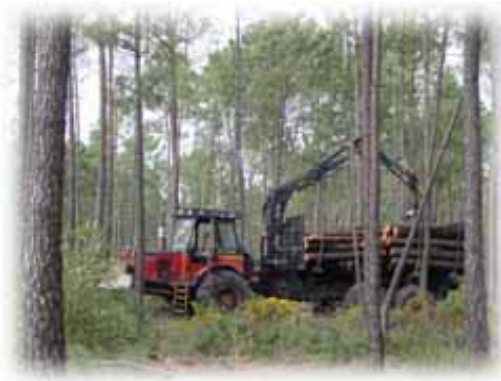
Figure 6-1: Forwarder working in the forest (source: www.logistica-florestal.pt ).
