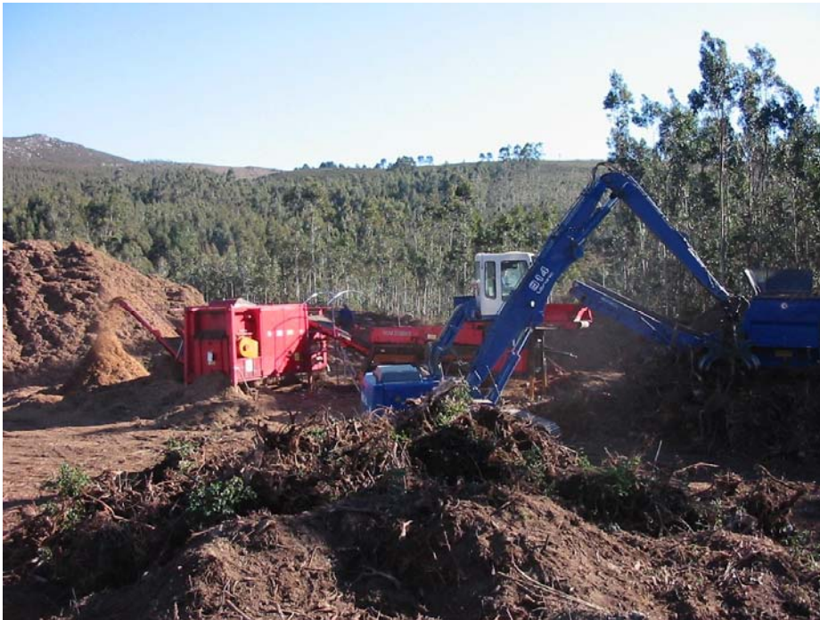
Figure 6-3: Harvester and wood chipper machines (source: Forestech).
