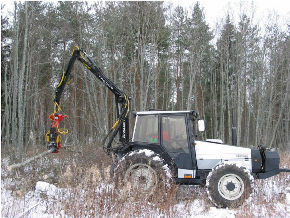
*Figure 1. EW harvesting contractor's farm-tractor attached with a crane and accumulating felling head.*
