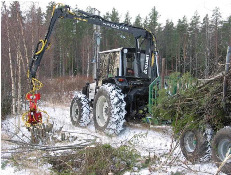
*Figure 4. Harvesting EW from the cartway side with farm-tractor based EW system.*
