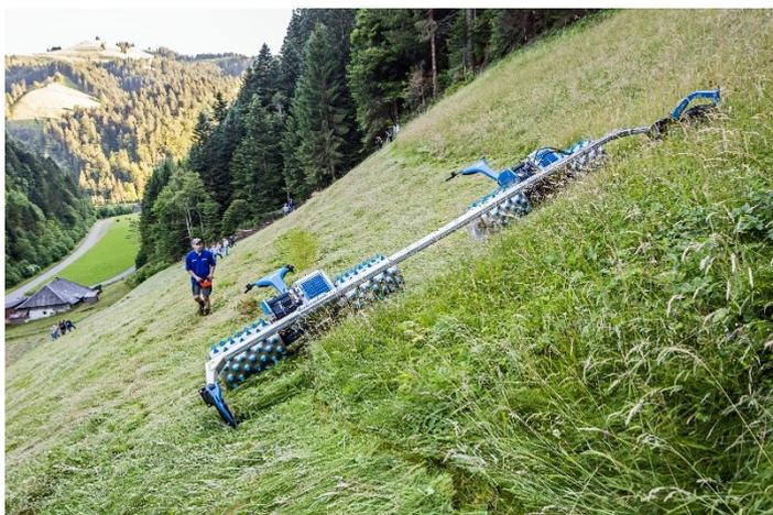
An innovative cutter bar mower with a working width of 6 m (Brielmaier). This machine is very effective and nature sensitive and therefore very suitable for HNV grasslands.
