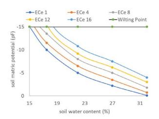
Figure 2: The effect of soil salinity (5 levels of soil electrical conductivity, ECe) on the relationship between soil potential ( $\Psi$ ) and soil water content
