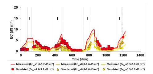
Figure 4: Electrical conductivity of the soil solution (EC) in soil lysimeters irrigated with different water qualities ( $EC_{iw}$ , electrical conductivity of the irrigation water; I, irrigation season) (Adapted from Gonçalves et al., 2006).
