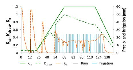
Figure 5: Evolution of the basal crop coefficient (Kcb), actual basal crop coefficient (Kcb act), and evaporation coefficient (Ke) in irrigated maize grown under saline conditions in southern Portugal (modified from Rosa et al., 2016).
