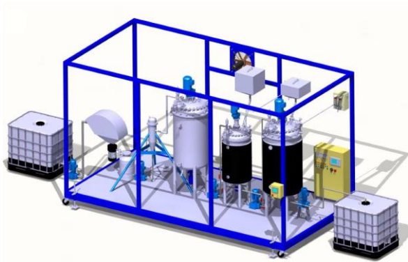
Fig. 2: Container plant for anaerobic digestion
