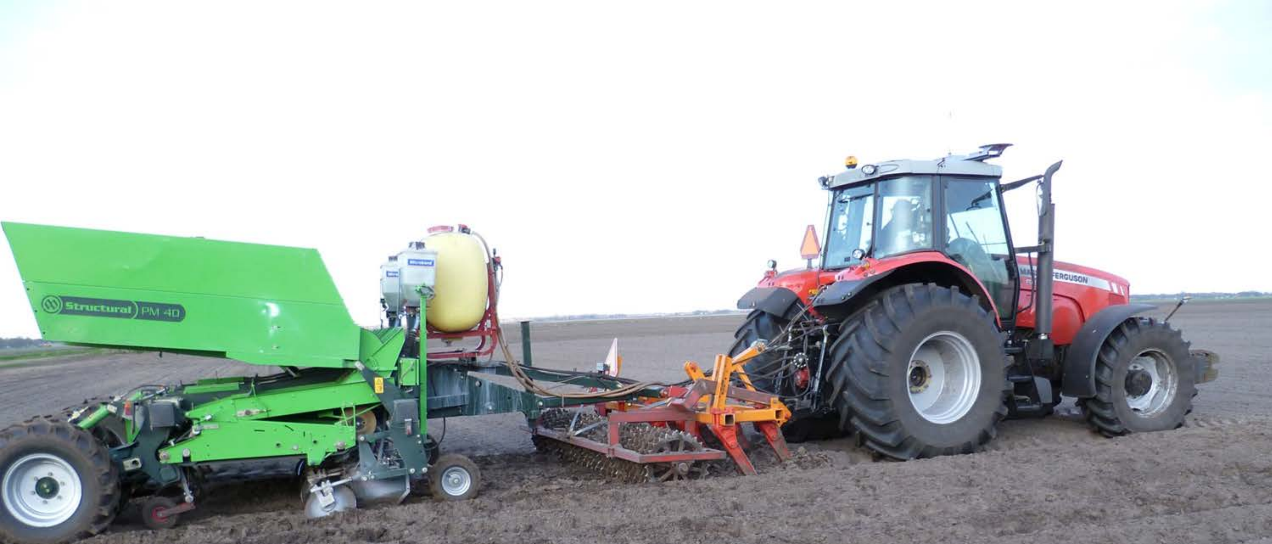
Integrated soil preparation and potato planting
