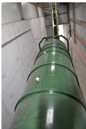
Figure 3. Aerated drum for biothermal drying on farm scale level
