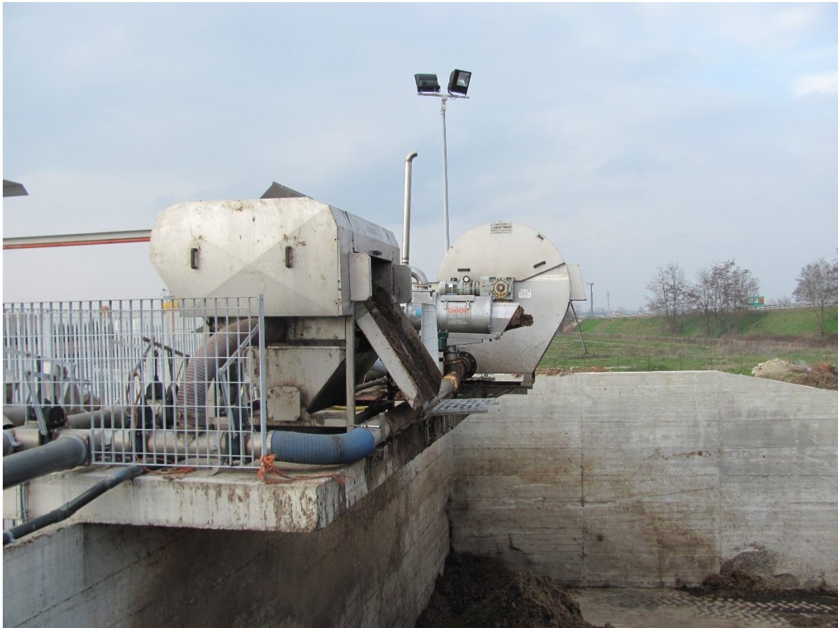
Figure 4. slurry separation devices used at farm scale (belt press and screw press)
