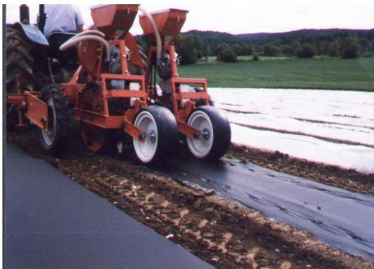
**Figure 1.** The laying of biodegradable mulching film in the field (BioBag, 2020).
