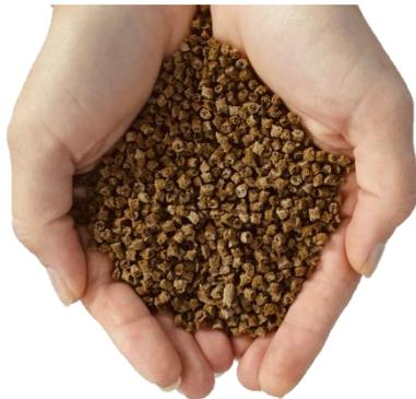
**Figure 10.** Biocomposite formulation from hop waste residues developed by TECNOPACKAGING (LIFE BioTHOP, Photo: Žepič Bogataj, V.)
