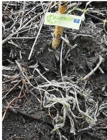
**Figure 8.** Testing the composting of bio degradable twine for its further use in bean production. Picture after 11 weeks of composting (LIFE BioTHOP PLA twine, 2020, Photo: Čeh, B.)
