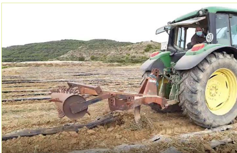
Figure 12: Tool to remove plastic mulch from the field with a tractor. The plastic mulch should be thick and strong enough to resist the removing process.
