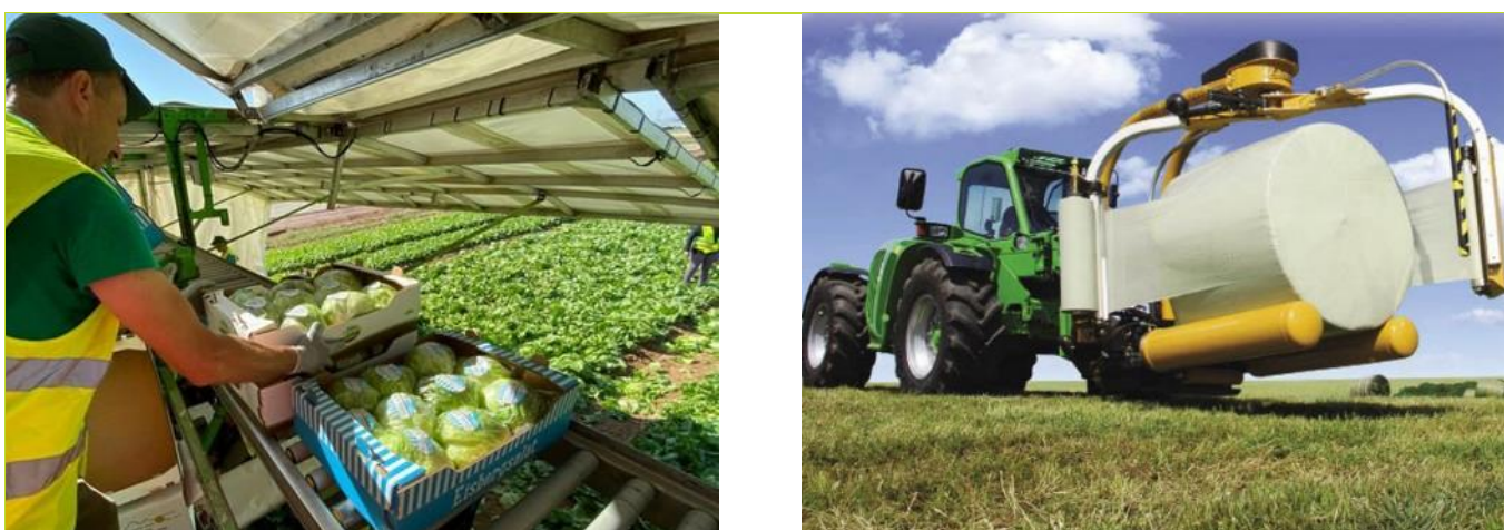
Figure 2: Examples of plastic films used in agriculture: Lettuce being wrapped in plastic in a harvesting mobile station (left – copyright www.hortidaily.com), bale being wrapped in plastic for silage preparation (right – copyright www.farm-equipment.com)
