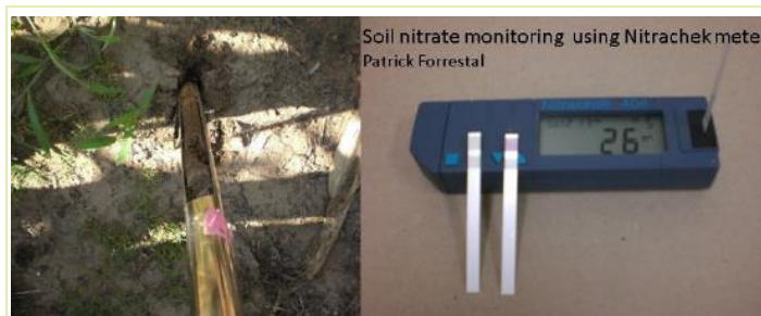
Figure 2. A quick test is used to measure soil nitrate; in the future, the development of smart sensors may make real-time monitoring of soil nitrate levels easier.
