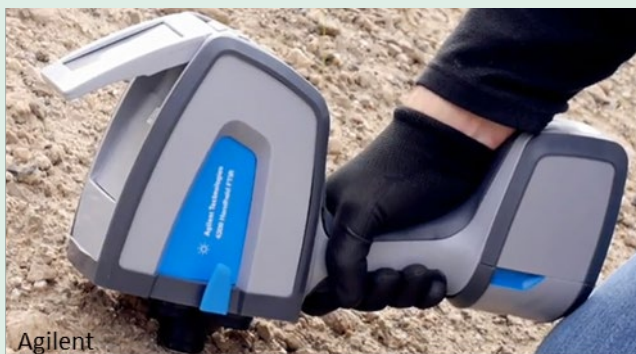
Figure 9. Handheld FTIR could enable the assessment of microplastics in the field.
