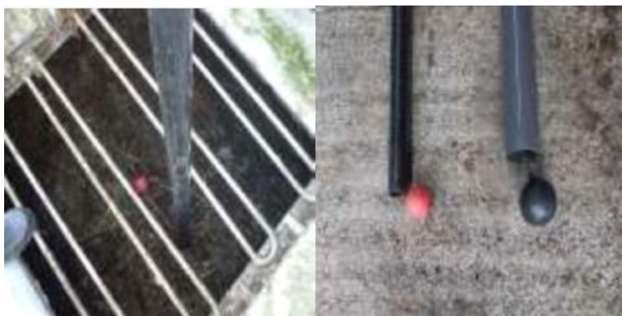
Figure 1: 'tube sampler' method
