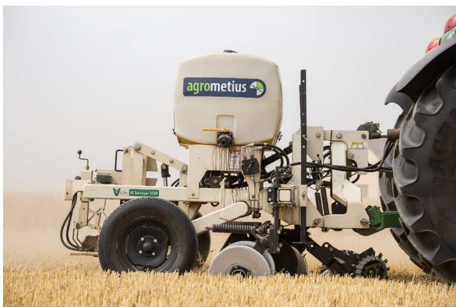
Figure 4: Soil scanner with 'Veriscanner'
