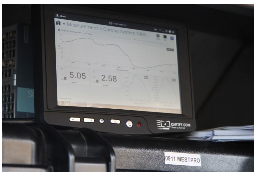
Figure 3: Output manure composition by measurement with NIRS-sensor (source: VCM, 2015)
