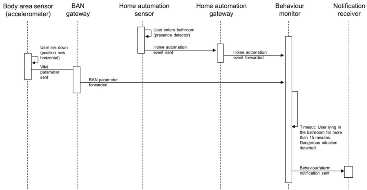
High level process flow - example 3: fall detection
