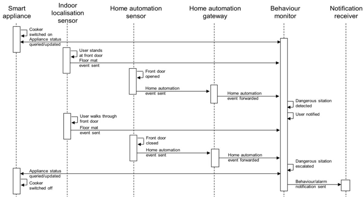
*High level process flow - example 1: dangerous situation detected using home automation sensors*
