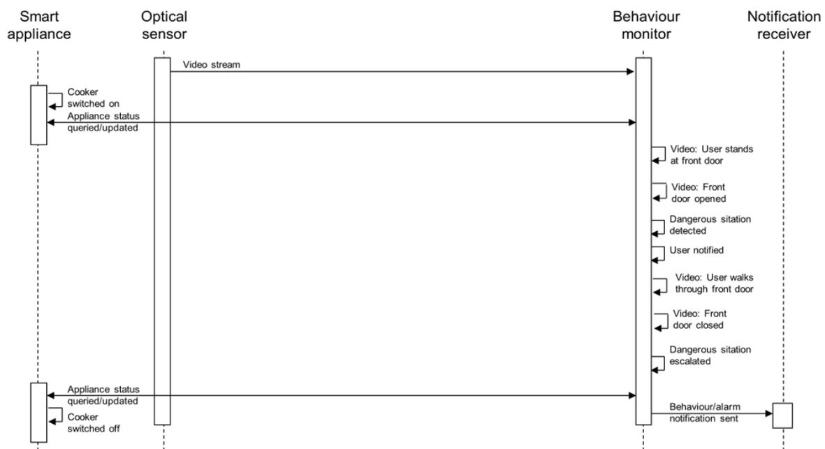
*High level process flow - example 2: dangerous situation detected optical sensors*
