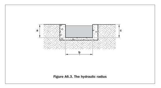
A completely filled, rectangular, smooth concrete drain of 1.5 m by 0.7 m, with a gradient of 0.005, can in ideal circumstances discharge around (1000 x ((1.5 x 0.7) x ((1.5 x 0.7/(1.5 + 0.7 + 0.7))^{0.67} x (0.005)^{0.5}) / 0.015) = 2500 litres per second.
