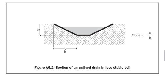
the hydraulic radius is the surface area of the cross section of the flow/the total length of the contact between water and drain;
