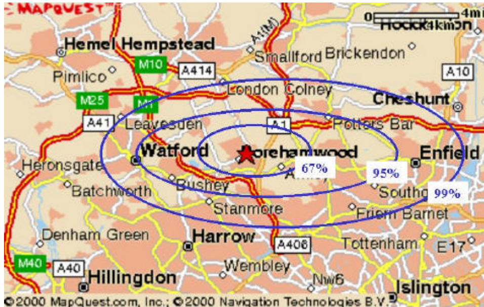
Figure 1: the star represents the estimated position. The percentage indicates the likelihood of finding the user in the area.
