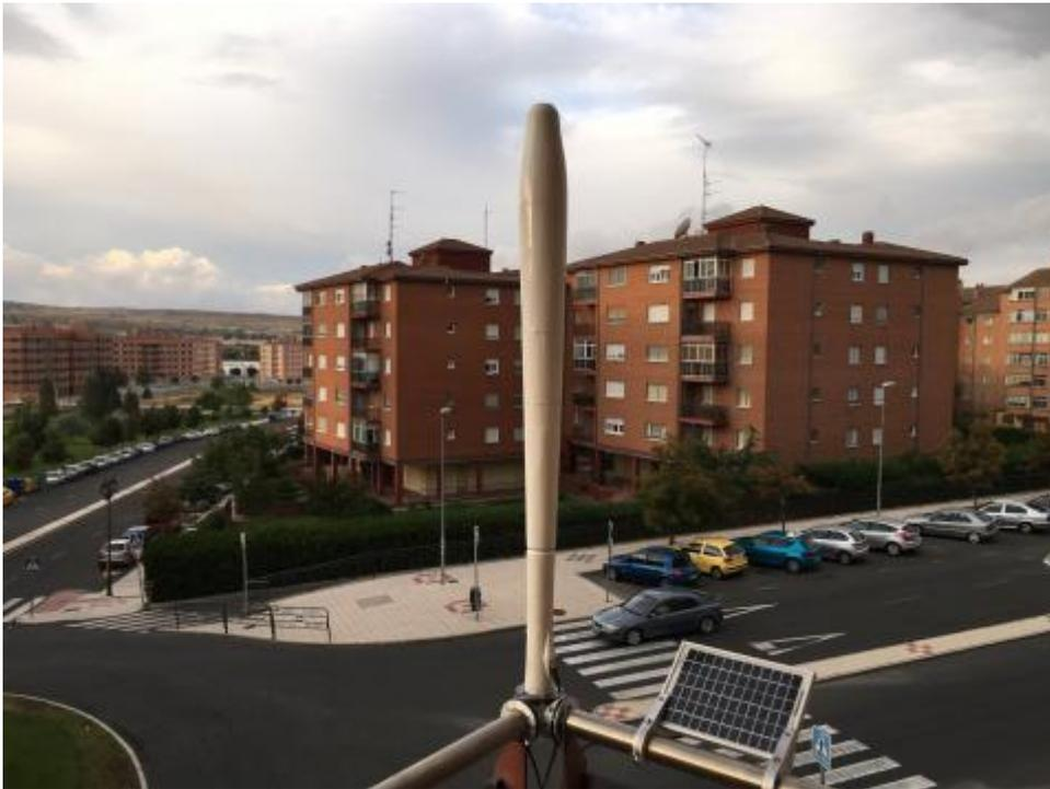
What's the common link between migrating birds, a collapsing bridge and a windmill? The answer is a bladeless wind turbine. Vortex Bladeless converts a natural wind phenomenon, which led the Tacoma Narrows Bridge to sway and break in 1940, into renewable energy. The turbine works without blades, saving migrating birds from sudden collision.
