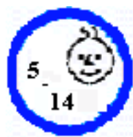
Figure 5.2: Warning symbol : luminaire adapted to a category of children
