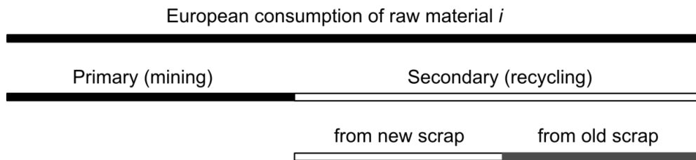
Figure 50: Schematic representation (not to scale) of recycling as included in the EU criticality exercise: only recycling from old scrap is considered in the calculation of supply risk.
