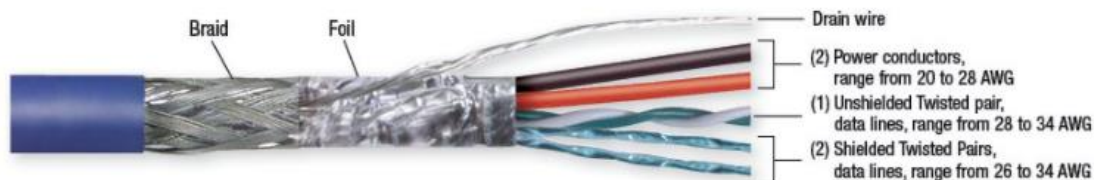
Figure 11. Example of USB 3.0 cable composition
