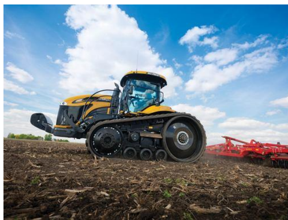
Figure 2. AGCO Challenger MT700 series (5 track roller pairs per track unit. 10 roller pairs per vehicle)
