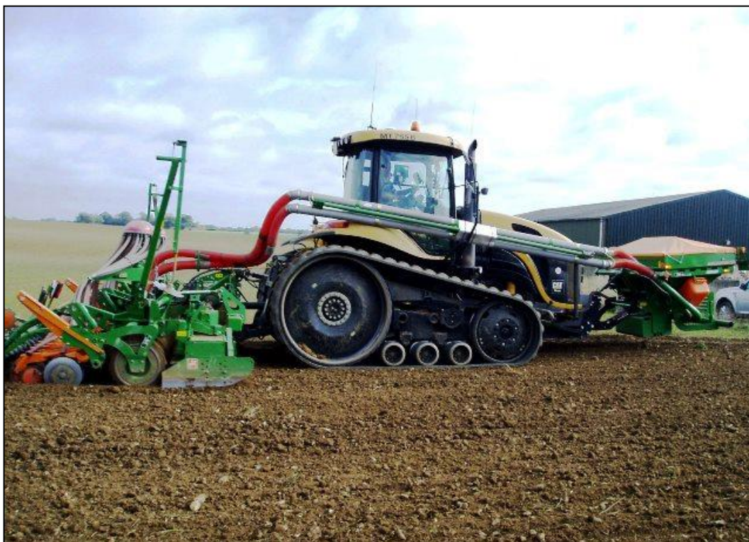
Figure 3. AGCO Challenger MT700 series plus 6 metre power-harrow drill combination and front-mounted 2000 litre seed hopper. In transport ( top ) and in-work ( below ) (Tractor mass ~ 15,000 kg, rear implement ~ 5,500 kg, front hopper ~ 2,500 kg: Total ~ 23,000 kg, Vehicle max. permissible mass ~19,000 kg)
