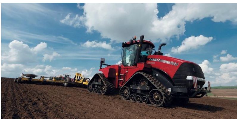
Figure 1. Case IH Quadtrac (5 track roller pairs per track unit. 20 roller pairs per vehicle)
