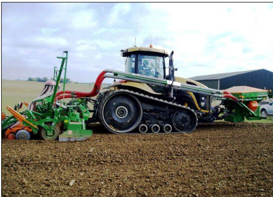
Figure 3. AGCO Challenger MT700 series plus 6 metre power-harrow drill combination and front-mounted 2000 litre seed hopper. In transport ( top ) and in-work ( below ) (Tractor mass ~ 15,000 kg, rear implement ~ 5,500 kg, front hopper ~ 2,500 kg: Total ~ 23,000 kg, Vehicle max. permissible mass ~19,000 kg)
