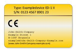
Template of a correct data plate for an importer (instead of a name a registered trade mark could also be used):
