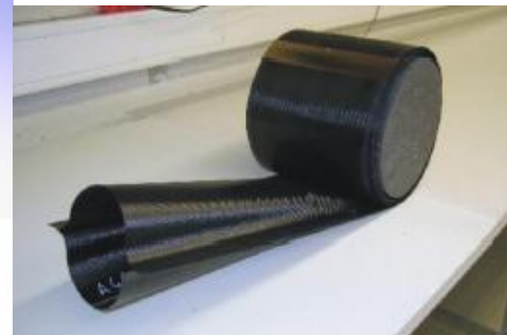
Below: Detail of 'lenticular' boom section
