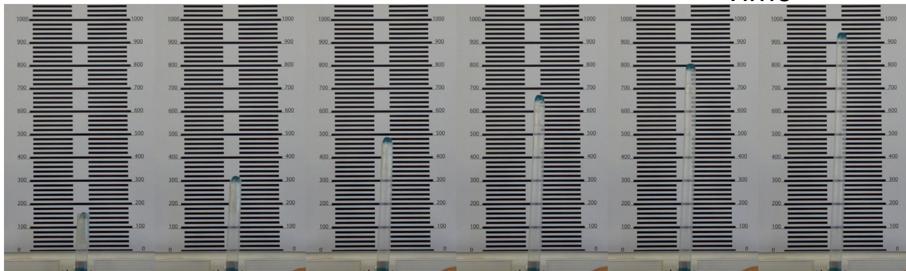
Above: Conical folding pattern (exaggerated taper) Below: Inflation test on a lightly tapered polymer boom
