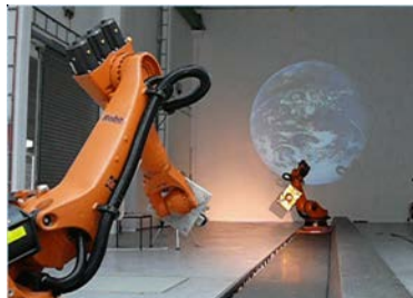
Test bed for approaching and docking
