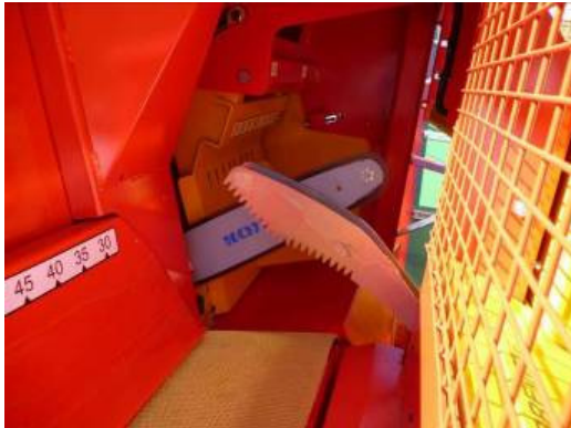
Figure 3 Log gripper near chainsaw
