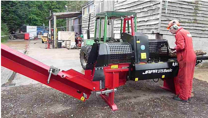
Figure 1 Tractor Power take off (PTO) shaft driven professional Firewood Processor
