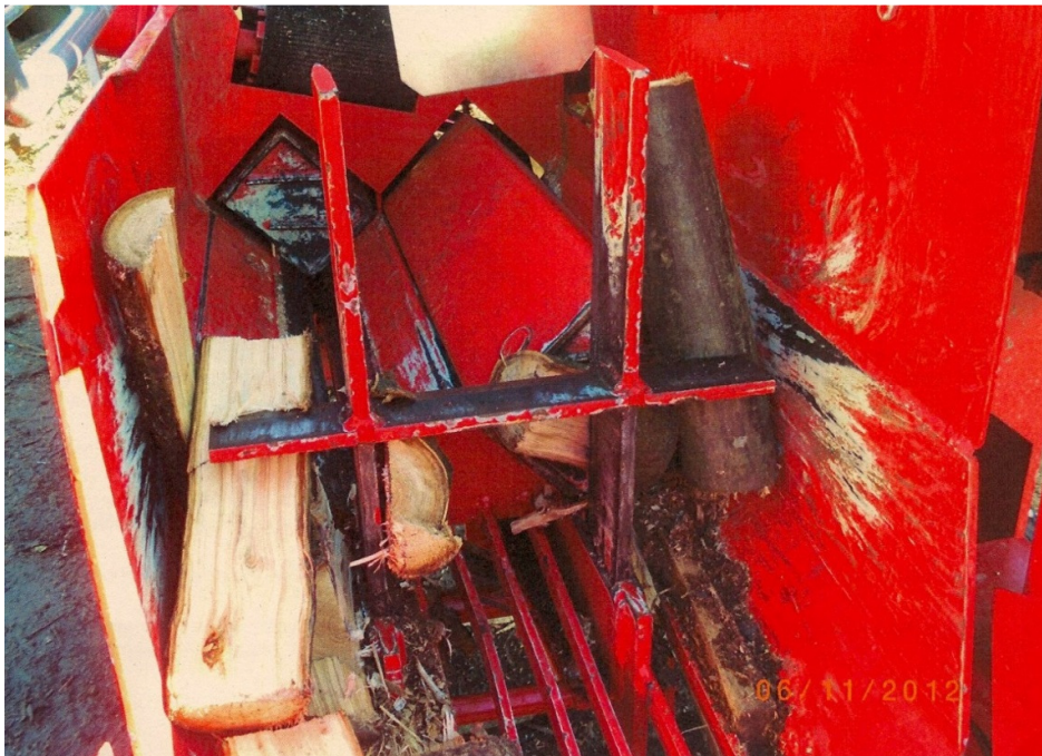
Figure 5 Logs jammed around splitter (here a six-way splitter with double rams)
