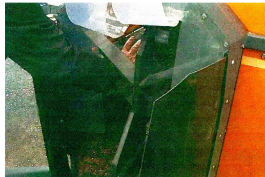
Figure 6 Flap 'guard' on splitter discharge and easy hand reach to splitter cutting edge
