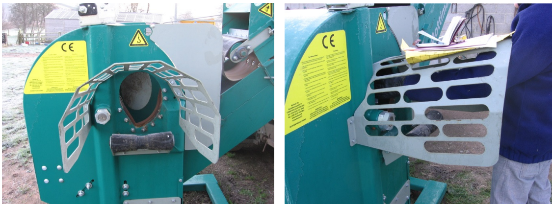
Figures 9 & 10 In-feed guard & support roller, easy access to rotating spike/blade!
