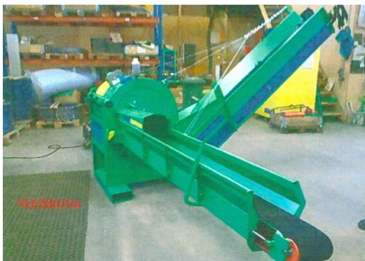
Figure 13 In-feed conveyor with tunnel guard
