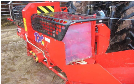
Figure 6 Flap 'guard' on splitter discharge and easy hand reach to splitter cutting edge
