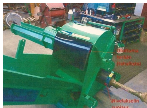
Figure 14 'Flap' on entry to discharge Conveyor not prevent access to danger
