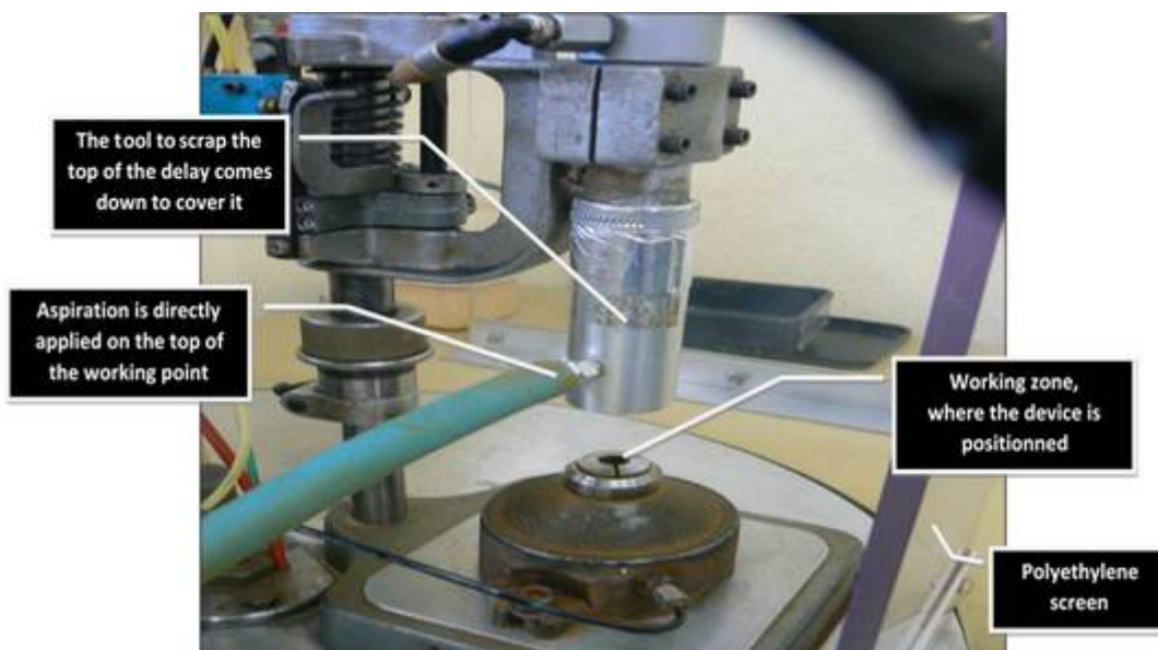
Figure 8: Photograph of the management measures for the delay scraping operation (ES-3 / Worker contributing scenario 1).
