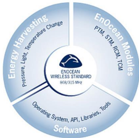
Source: EnOcean website - EnOcean Dolphin System Architecture 11
