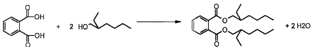
Figure 2.3: Production of Di (2-ethylhexyl) Phthalate
