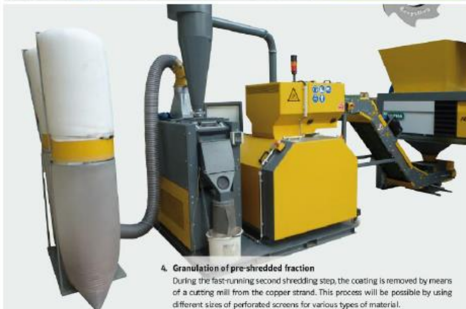
Figure 3-21: Detailed process flow of cable waste shredding 95 .
