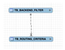
Routing criteria contains the data that are needed to perform the routing of the messages to a specific plugin implementation.
