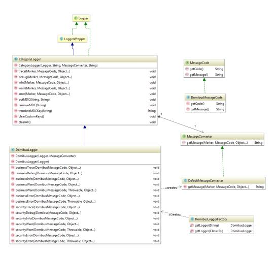
There are three types of logs: security logs, business logs and miscellaneous logs. Each log category has its own marker defined in the DomibusLogger class. By default, each category will be logged in a separate file:
