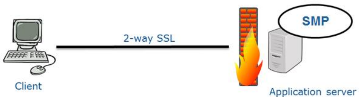
Figure 14 2-way-TLS scenario with truststore configured within J2EE container
