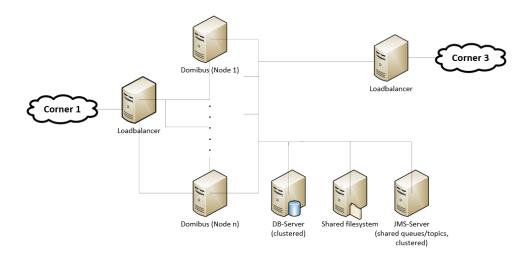
It is important to note that not all physical nodes are represented on this diagram. Indeed load balancers, database servers and JMS servers could be duplicated for scalability, performance and availability reasons. Furthermore, security mechanisms like firewalls are not shown.
