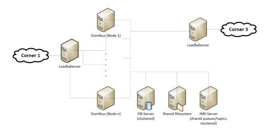
It is important to note that not all physical nodes are represented on this diagram. Indeed load balancers, database servers and JMS servers could be duplicated for scalability, performance and availability reasons. Furthermore, security mechanisms like firewalls are not shown.
