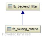
Routing criteria contains the data that are needed to perform the routing of the messages to a specific plugin implementation.
