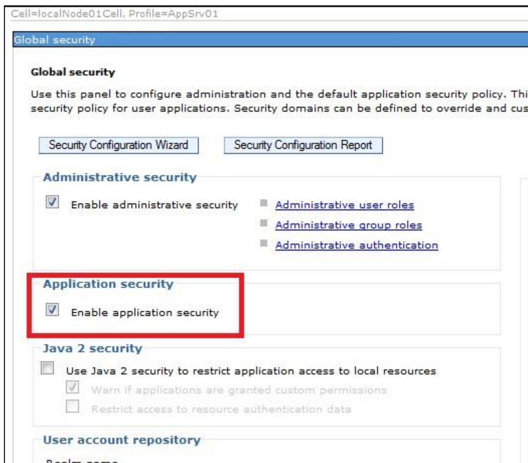
Figure 1: Enabling application security on WebSphere AS
