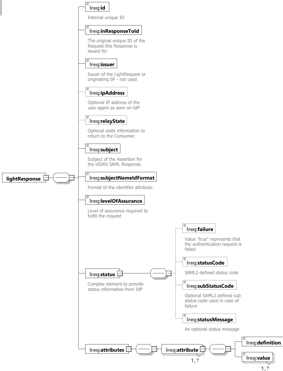
Figure 14: Simplified XML LightResponse schema
