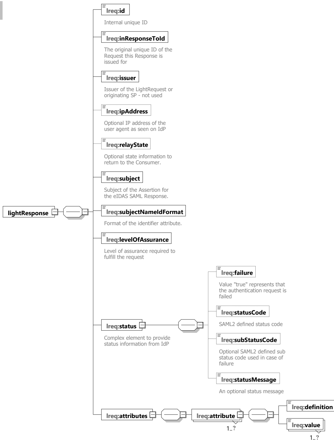
Figure 14: Simplified XML LightResponse schema
