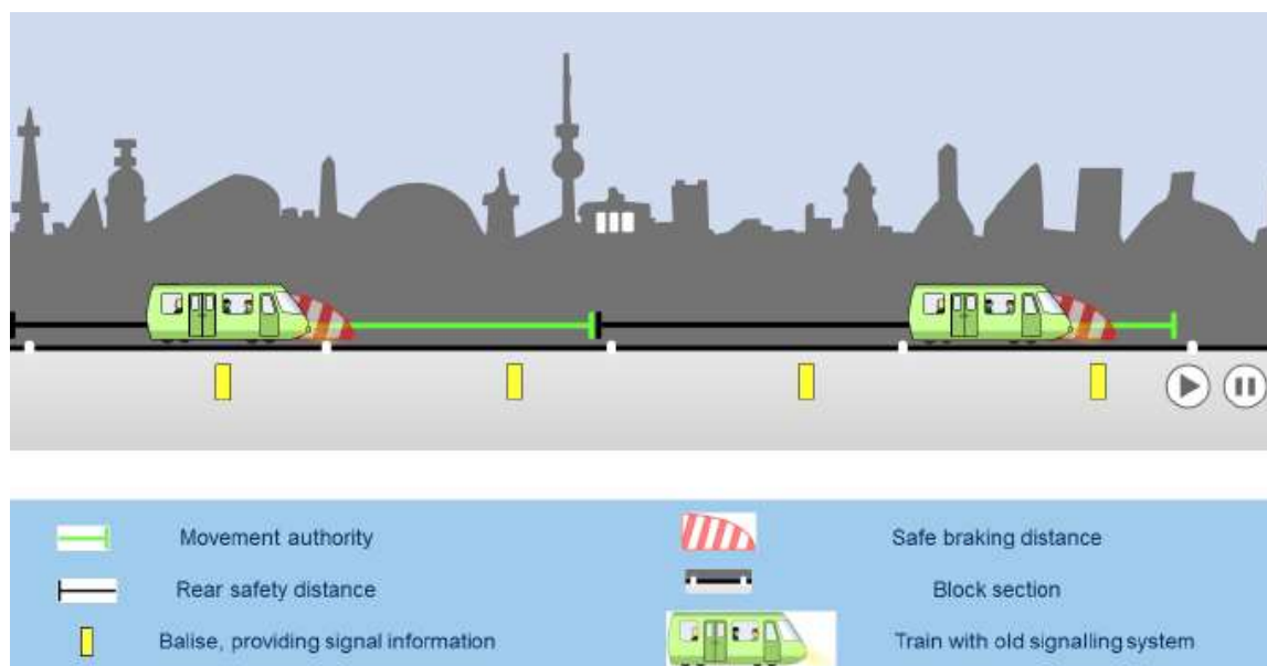
Figure 3: Urban signalling (Metro) – Conventional technology
