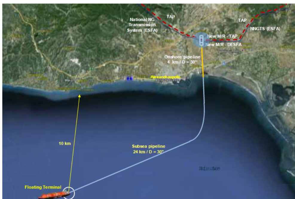
Figure 2: Pipeline and connection to NNGTS
