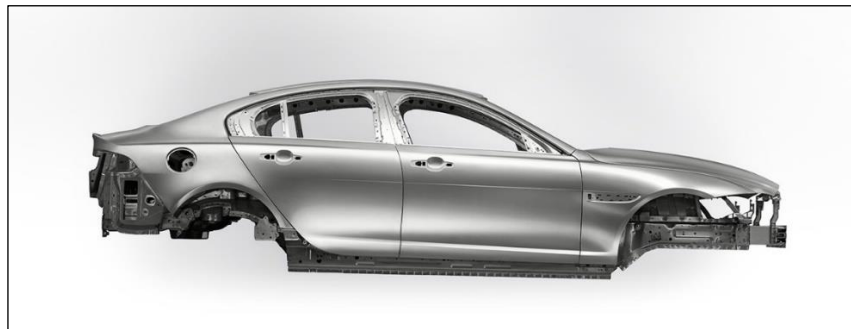
Figure 2 An example of aluminium body-in-white (Jaguar XJ)
