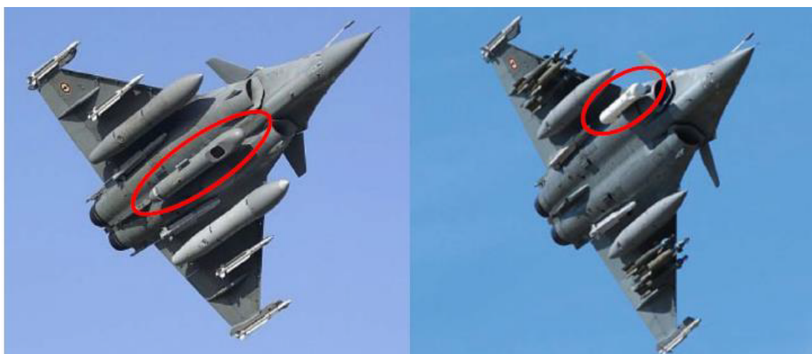
Figure 6: Dassault's Rafale jet fighter carrying a podded EO/IR sensor for reconnaissance (left) and a podded EO/IR sensor for targeting (right)
