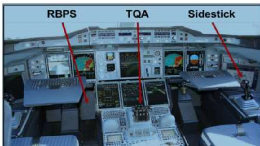
Figure 4 - Pilot controls in a cockpit
