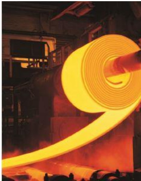
Figure 5 – HR coil exiting hot strip mill
