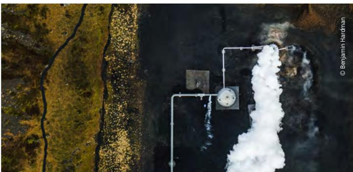
CO<sub>2</sub> dissolved in water is injected into underground basalt rock formations
