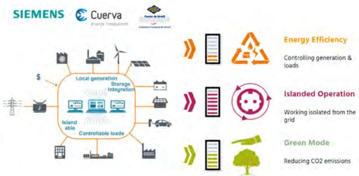
Microgrid of the Port. Controlled by the DEOP developed by Siemens, integrating all the data from several sources and devices.
