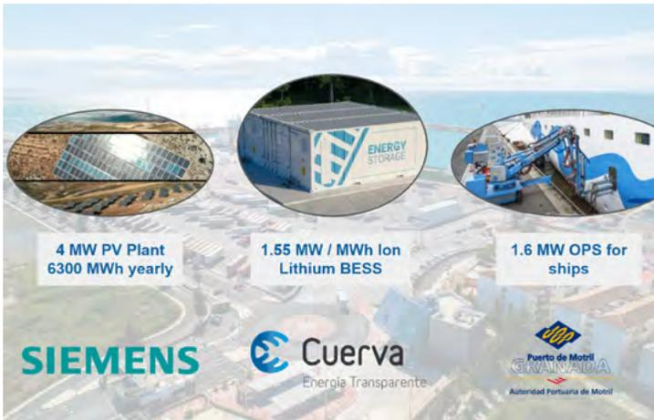
GREENMOTRIL seeks the energy independence from the Port of Motril by deploying on-shore renewable technologies
