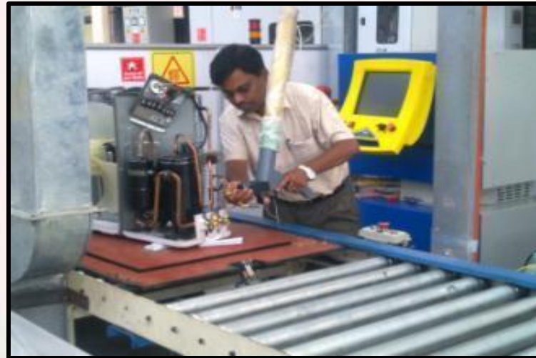
Gas charging station with ventilation ducting & gas alarms
